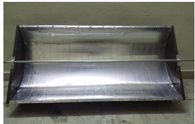
Fig. 2: Reflector with Al absorber tube
